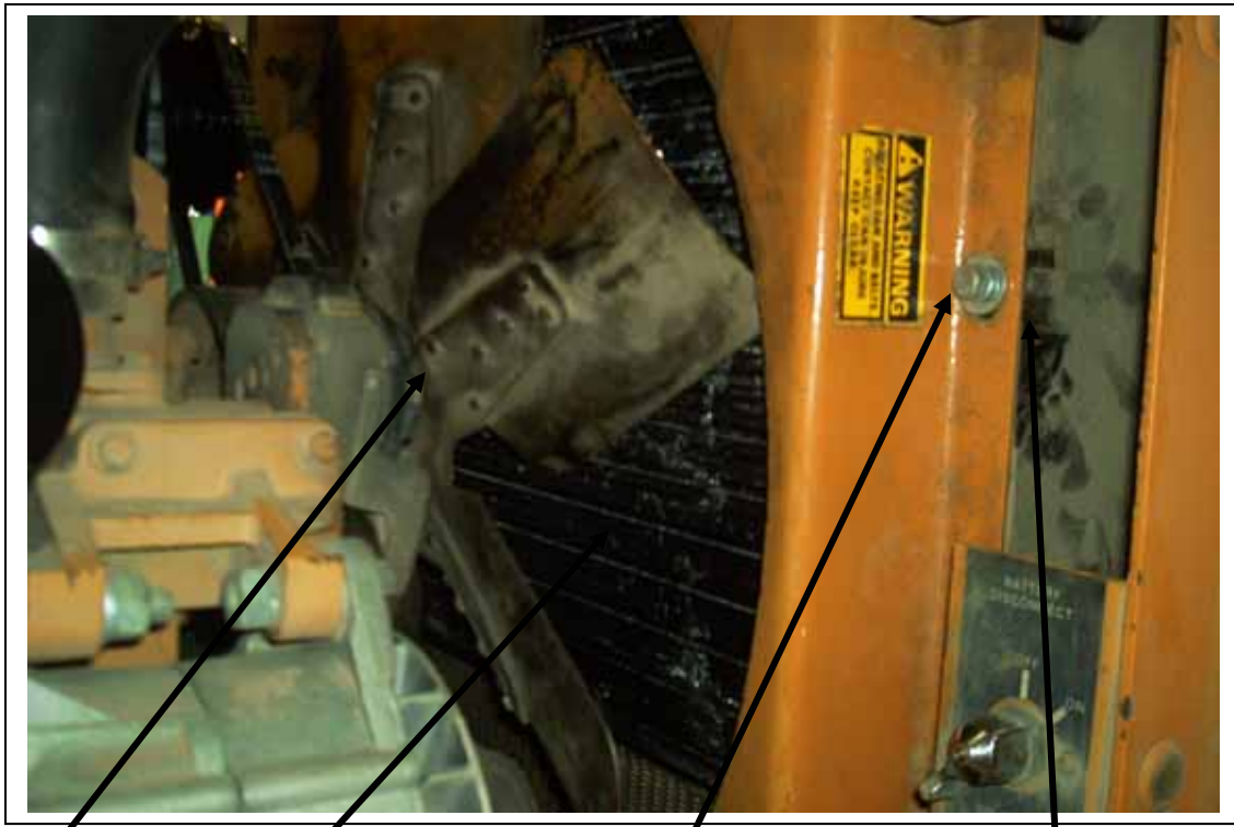
Fan Condenser Shroud mounting bolt. Slotted condenser bracket.
