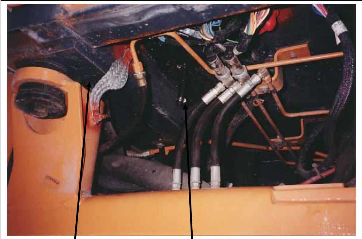
A/C hoses entering the cab
