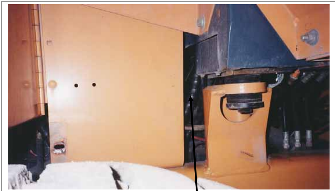
A/C hoses entering the cab
